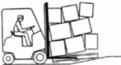
Ramps and bumpy floors can cause loads to be jolted and bases of pallets to be grazed.
